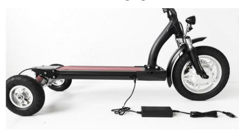
Note: please connect to the charging port of the electric scooter, connect with the socket, connect with the socket, and the red light will be on when the charger is connected.
